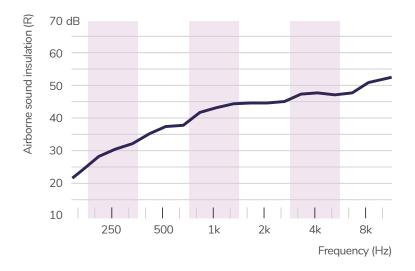
Sound insulation measurements on AFT door took place in a laboratory. Single leaf, size 1045 x 2235 mm, with threshold H=48 mm, 2 pcs compression type latches, no vision panel. Different leaf configuration, door size, threshold, locks, vision panels, etc. will affect sound insulation values.
