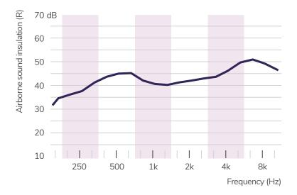
Sound insulation measurements on A43 door took place in a laboratory. Single leaf, size 950 x 2100 mm, with threshold H=48 mm, 2 pcs compression type latches, no vision panel. Different leaf configuration, door size, threshold, locks, vision panels, etc. will affect sound insulation values.
