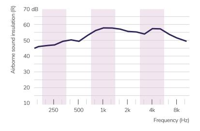
Sound insulation measurements on A56L door took place in a laboratory. Single leaf, size 950 x 2100 mm, with threshold H=48 mm, 2 pcs compression type latches, no vision panel. Different leaf configuration, door size, threshold, locks, vision panels, etc. will affect sound insulation values.
