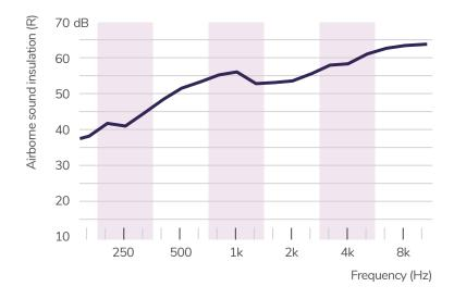
Sound insulation measurements on A53 door took place in a laboratory. Single leaf, size 950 x 2100 mm, with threshold H=48 mm, 2 pcs compression type latches, no vision panel. Different leaf configuration, door size, threshold, locks, vision panels, etc. will affect sound insulation values.
