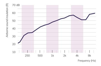
Sound insulation measurements on A51 door took place in a laboratory. Single leaf, size 950 x 2100 mm, with threshold H=48 mm, 2 pcs compression type latches, no vision panel. Different leaf configuration, door size, threshold, locks, vision panels, etc. will affect sound insulation values.
