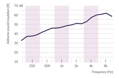
Sound insulation measurements took place in a laboratory. Specimen door A47, single leaf, size 950 x 2100 mm, with threshold H=48 mm, 2 pcs compression type latches, no vision panel. Different leaf configuration, door size, threshold, locks, vision panels, etc. will affect sound insulation values.
