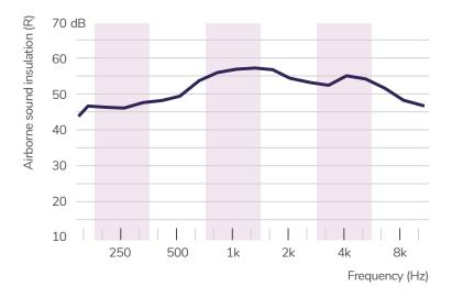
Sound insulation measurements on A55L door took place in a laboratory. Single leaf, size 950 x 2100 mm, with threshold H=48 mm, 2 pcs compression type latches, no vision panel. Different leaf configuration, door size, threshold, locks, vision panels, etc. will affect sound insulation values.
