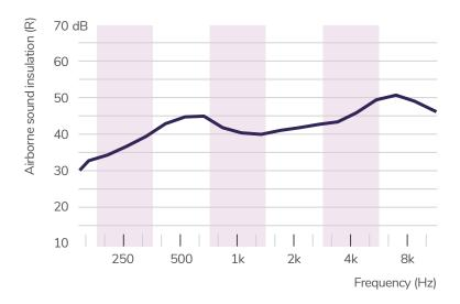
Sound insulation measurements took place in a laboratory. Specimen door A41, single leaf, size 950 x 2100 mm, with threshold H=48 mm, 2 pcs compression type latches, no vision panel. Different leaf configuration, door size, threshold, locks, vision panels, etc. will affect sound insulation values.
