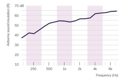
Sound insulation measurements on A52 door took place in a laboratory. Single leaf, size 950 x 2100 mm, with threshold H=48 mm, 2 pcs compression type latches, no vision panel. Different leaf configuration, door size, threshold, locks, vision panels, etc. will affect sound insulation values.
