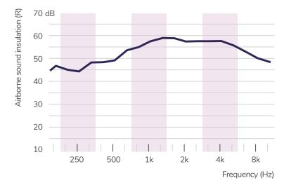
Sound insulation measurements on A56 door took place in a laboratory. Single leaf, size 950 x 2100 mm, with threshold H=48 mm, 2 pcs compression type latches, no vision panel. Different leaf configuration, door size, threshold, locks, vision panels, etc. will affect sound insulation values.
